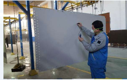
Enamel Thickness Test
